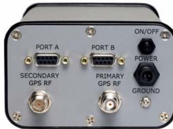
Figure 4-1. Turn the Crescent VS100 on at the Power toggle switch.
