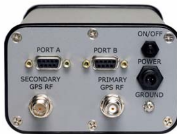
Figure 3-4. Port connections on the Crescent VS100.
