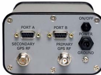
Figure 5-1. Turn the Crescent VS100 on at the Power toggle switch.
