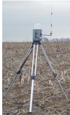
Figure 4-1. Base station on tripod
