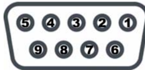
Figure 3-5. DB9 female socket numbering
